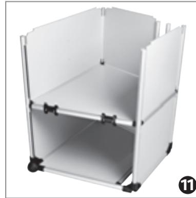
Insert the remaining two back panel profiles (A) into the connectors and add the second base plate, the second back panel and the second top plate.
