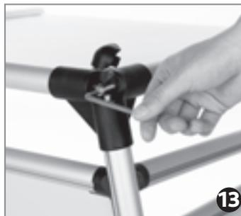
Tighten all the screws, including the ones you have loosened, step by step going round from corner to corner. When everything has been screwed together tightly, all parts will be in their final position, and the 1–1.5 cm gaps between connectors and lattice bars close. To achieve a straight result without gaps it is vital to tighten the screws step by step and evenly on all sides. At the end all screws should be securely tightened.
