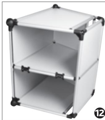
Last add the left side panel. For this press all four corners down evenly and with force. It is normal that the transport box is under high tension for this step. This is necessary to prevent rattling when you are driving later. If you cannot fit this last panel correctly, it might be helpful to loosen the pre-mounted screws of this panel at the corners.
